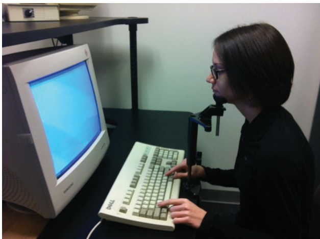
Fig. 1. A typical setup for studying perception. Chin rests are used to minimize head movements.
